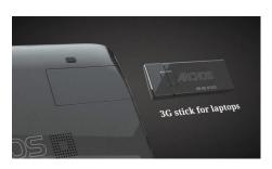
The G9 tablets feature a unique 3G ready solution where customers no longer need to choose between WiFi and 3G models at purchase. ARCHOS 9 3G Stick is a standard 3G stick for laptops which has been designed to be compatible with all ARCHOS G9 tablets. The ARCHOS G9 3G Stick has been specially designed to fit perfectly into the back of any G9 tablet. Just remove the cover and slide in the G9 3G stick. With no
